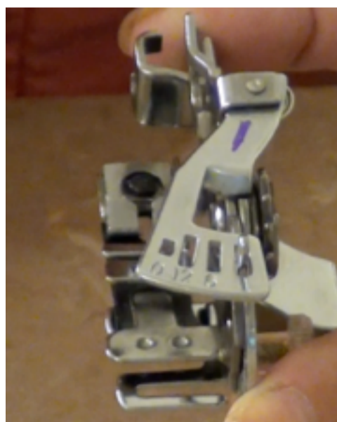
Adjusting lever takes a stick every 1, 6, 12 or 0 stitches
