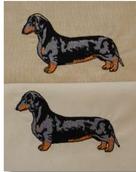
The registration problem on the upper design was caused by rotating the fabric 90°.
