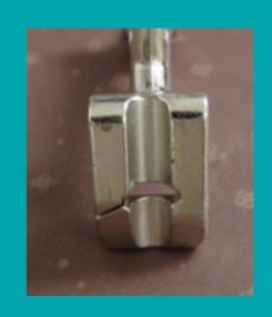
This foot has a groove on the underside of it The pearls, piping etc glide under the foot without touching it and are quickly attached to your project.
