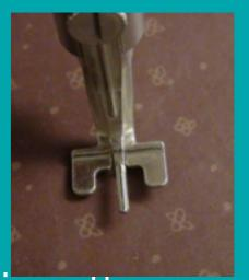
This foot holds your button in place while sewing the button on by machine, and it creates a shank for your button also
