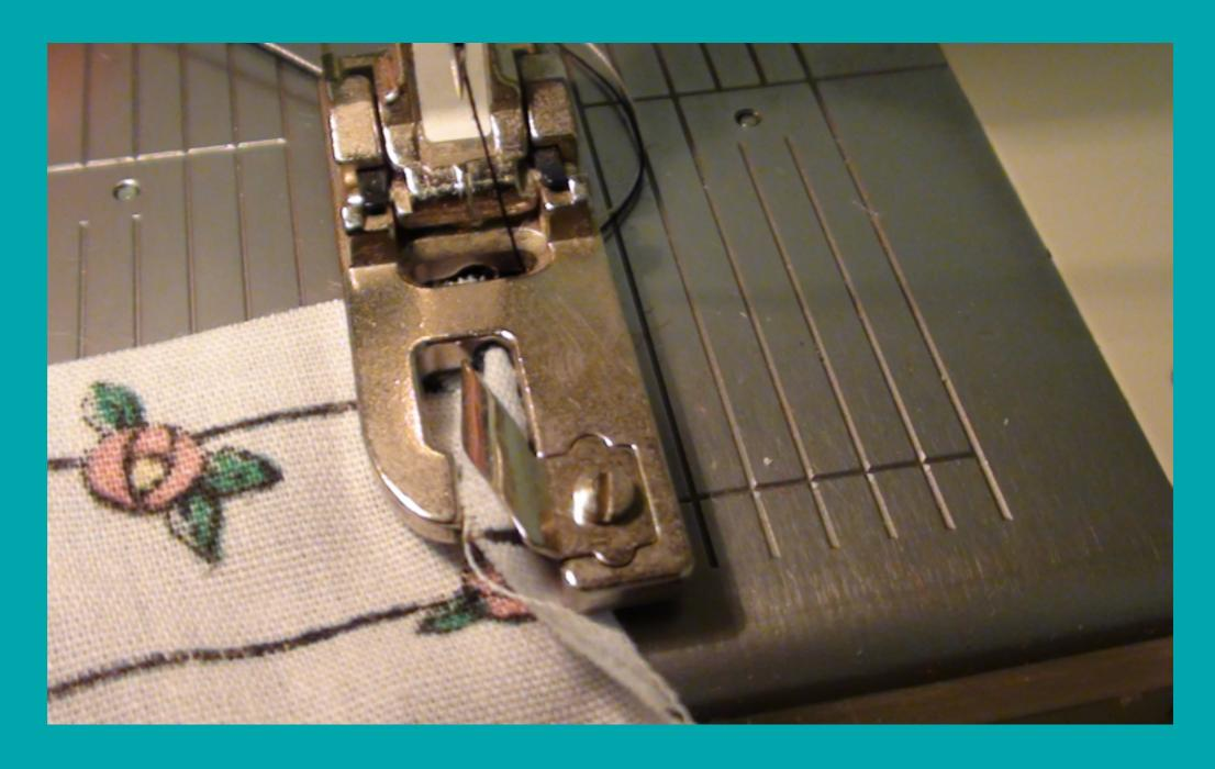
Completely fill the opening in the front of the foot with fabric but be sure there is no excess.
