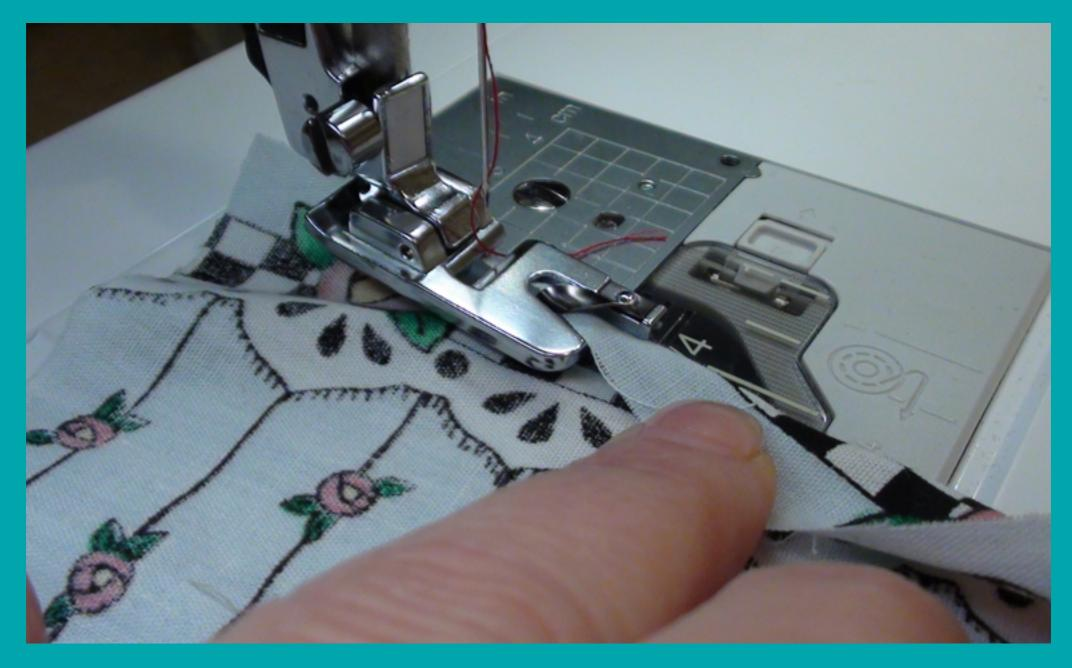
Put your fabric wrong side up under the foot and maneuver the fabric so it goes around the guide
