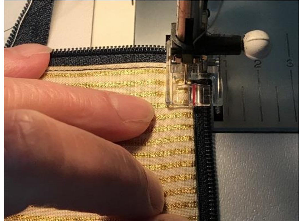
Align the mark on the foot with the folded edge of the square. Move the needle to the left if necessary.
