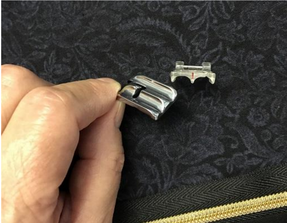
Double Welting Foot has 2 grooves
